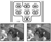
If the slow-motion playback continues for approx. 10 minutes or more, then the playback will automatically stop. (10 minutes of slow-motion playback is equivalent to approx. 2 minutes in the SP mode or approx. 3 minutes in the LP mode.)
