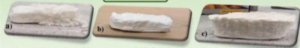
Figure 2 : Comparison of the appearance of cellulose foam a) unprocessed and b) cellulose foam processed with super masscolloider at 3 \times 150 \mu\text{m} & 3 \times 100 \mu\text{m} and c) cellulose foam processed at 5 \times 100 \mu\text{m} & 5 \times 50 \mu\text{m} & 5 \times 10 \mu\text{m} .
