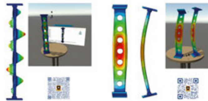
Local buckling in FEA vs Local buckling in MR
