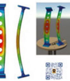
Overall buckling in FEA vs Overall buckling in MR
