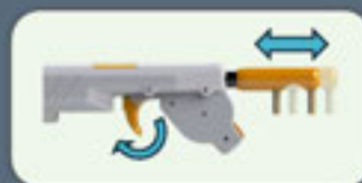
Pulling the trigger, the shaker head oscillates the blueberry cluster, shaking the berries off
