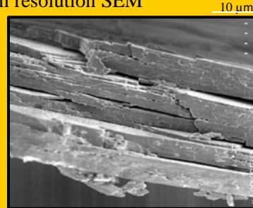
Figure 1. Anomiidae 600 °C at 4k magnification. 20 µm
