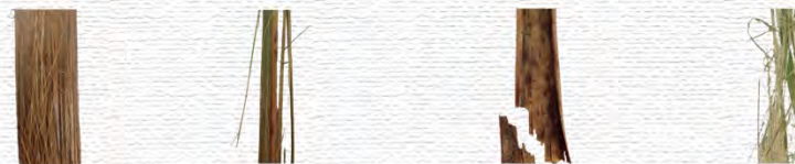
The images above are of samples pulled on until failure, from left to right, dried Tī kōuka, fresh Tī kōuka, dried Harakeke and fresh Harakeke.
