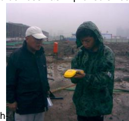
Using a Trimble GeoXT rugged handset for data acquisition and design at a Shanghai construction site.
